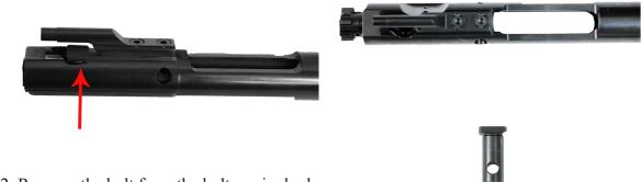
12. Remove the bolt from the bolt carrier body.
