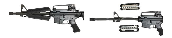
With the handguards out of the way, be certain not to distort or damage the gas tube.
