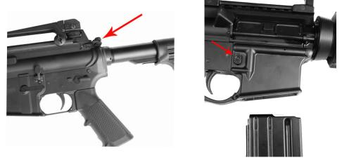
4. Remove the ammunition source by removing the magazine. To do so, depress the magazine release button and pull the magazine out the bottom of the magazine well.
