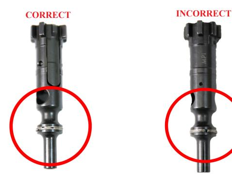
Correctly Staggered Gas Rings
