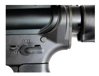
3. After one minute, unload the firearm per the directions noted under "Unloading Your Firearm" and inspect the primer on the live round that did not fire. Evaluate whether it is just a bad primer or if the primer was adequately struck by the firing pin. A light firing pin strike on the primer may be a result of a damaged or worn firing pin, a dirty firing pin chamber, or a broken firing pin spring.
