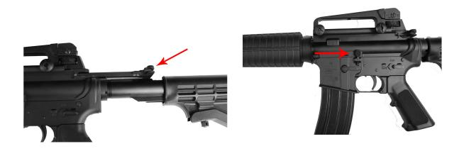
2. Push the charging handle forward until it snaps back into position.
