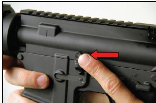
**5.** With selector pointing toward SAFE, return the bolt forward into battery by pressing the upper portion of the bolt catch.
