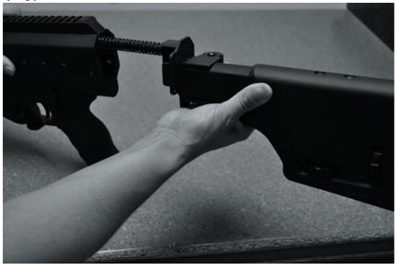
• Pull the charging handle gently to the rear and, before reaching the back of the charging handle slot, slide the handle out of the dovetail in the bolt carrier, removing it from the weapon. The charging handle is retained in position by the action springs.
