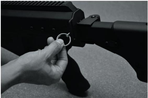
• Carefully pull out the butt stock with the receiver end plate assembly from the back of the rifle. This will also remove the action springs. Exercise caution as this part is under spring pressure.
