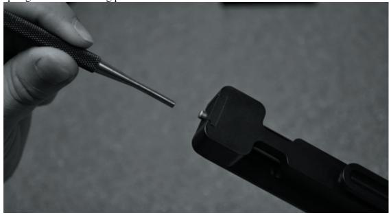
• Carefully allow the firing pin spring to relax, then tilt the bolt to remove the firing pin and the return spring.
