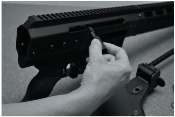
• Insert the charging handle in front of the carrier to slide the bolt and carrier assembly to the rear so that it extends beyond the back of the receiver and and can be grasped for removal.
