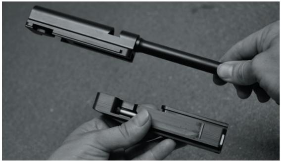
• Using a small punch or a 1/8 hex wrench, push the firing pin forwards against the spring until the retaining plate can be slid out.
