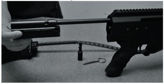
• With the bolt and carrier assembly removed, push the bolt backwards on the carrier to cam out the lugs. Note the lugs are not retained in place, so be careful to retain these to prevent them falling from the bolt.
