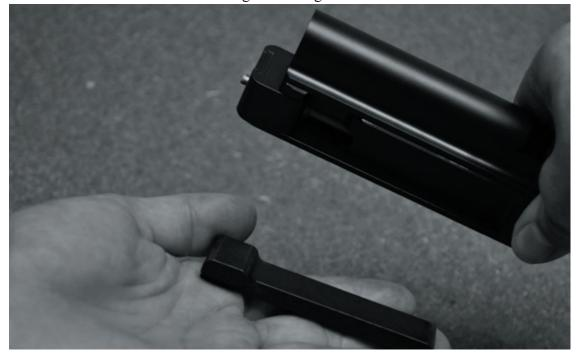
• The bolt can now be slid forward to fully remove it from the carrier.
