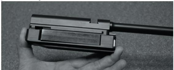
• Tilt the bolt to remove the left and right hand lugs.
