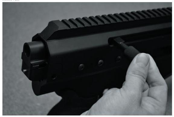
• Slide the bolt carrier assembly out of the rear of the receiver. The operating rod and piston will slide out with this assembly.
