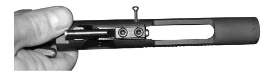
8. Tilt bolt face up and remove the firing pin.
