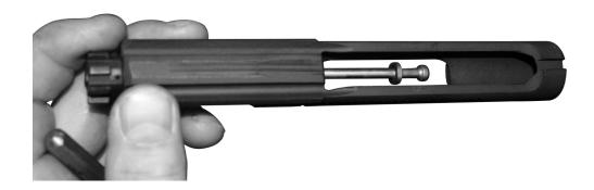
9. Push bolt in towards the carrier until it rotates and comes to a stop, then turn cam pin 90°.
