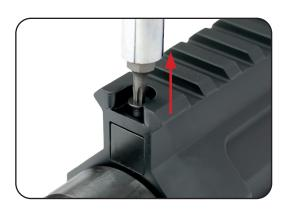
c. Hold the housing at a slight angle and remove the slide cover.
