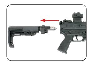
e. Separate the lower receiver from the weapon.
