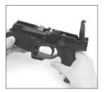
7. Slide the front of the lower receiver into the recess provided for it in the upper receiver and rotate the lower receiver up into the upper receiver until the retaining plate latches into the top of the upper receiver.
