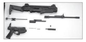
**NOTE:** The barrel can be removed without disassembling the rest of the rifle. To remove the barrel without disassembling the rest of the rifle pull the bolt handle back until the handle aligns with the marks on the receiver and pull it out and rotate the handle into the ejection port so that the bolt carrier assembly is locked in place. Then remove the barrel as stated in step seven (page 32).
