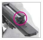
4. Slide the barrel into the receiver and press it into place. The barrel is seated when the barrel release levers snap up locking the barrel in place. Pull forward on the barrel after it is seated to make sure it is retained.
