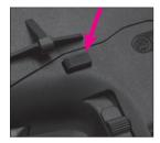
An alternant method of removing the magazine is to press up on the lower magazine release button located on the bottom of the trigger guard just behind the magazine well until the magazine is released then pull the magazine down and out of the rifle.
