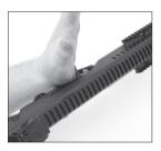
6. Rotate the safety selector lever to the disassembly position, depress the retaining latch on the back of the lower receiver and allow the safety to pivot back to the on position while holding the retaining plate forward. The retaining plate will be held slightly forward by the safety selector lever allowing it to clear the back of the upper receiver when it is installed.
