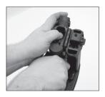
4. Pull down on the lower receiver while holding the safety lever in the disassembly position and depressing the retaining plate through the back of the receiver and remove the lower receiver from the upper receiver.
