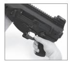
**NOTE:** The bolt carrier must be completely forward to allow the retaining plate to pass the recoil spring guide.
