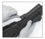
To reinstall the rail cover, slide the rail cover over the accessory rail and pull it back until the tab at the back of the rail cover snaps into the recess in the receiver.
