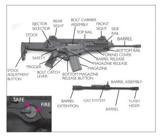
The Beretta ARX100 is a semiautomatic rifle that is designed to survive extreme environmental conditions and provide a modern, completely ambidextrous rifle that can be readily adapted to fit the largest number of users and be configured to suit situational requirements.
