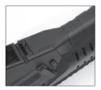
The grip of the ARX100 contains a storage compartment that can be used to store cleaning supplies, tools, small parts, batteries or accessories. To access the compartment press in on the button located on the bottom right side of the grip using a bullet tip or similar shaped tool and pull down on the ledge at the bottom back of the grip. The grip cap will pull out of the bottom of the grip exposing the compartment.
