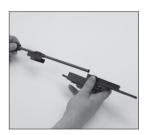
9. Remove the bolt from the bolt carrier by rotating the bolt handle to the right or left side (do not push the bolt handle into the bolt) and pull the bolt back through the bolt carrier rotating it to allow the bolt cam to follow the cam path and remove it from the carrier.
