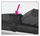
An alternate method of locking the bolt carrier assembly open is to insert an unloaded magazine and retract the bolt handle until the magazine follower pushes the bolt catch up, locking the bolt carrier assembly to the rear.
