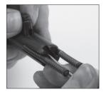
2. With the bolt handle moved to the left or right side, slide the bolt into the bolt carrier from the back with the cam pin aligned with the cam pin path until the bolt sticks out the front of the carrier then rotate the bolt handle to align with the length of the bolt.
