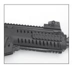
To remove the rail cover, pull up on the back of the rail cover slightly and slide it forward and off the forend.
