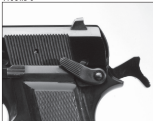
The hammer in the full-cock position.
