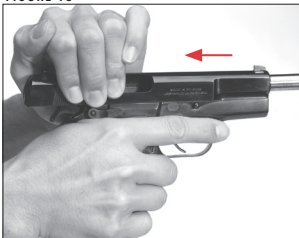
Pull the slide completely rearward and release it, allowing it to move forward freely.
