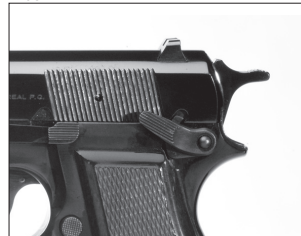
The hammer in the half-cock position.
