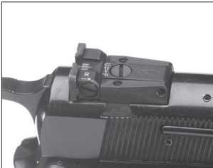
The adjustable rear sight can easily be tuned for windage (side screw) and elevation (top screw) corrections.
