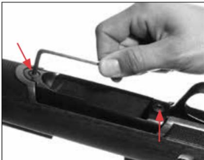
Remove the two screws and lift the bottom metal from the stock.
