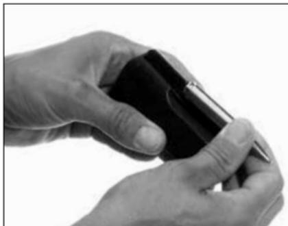
Depress the follower with the rim of the cartridge and slide the cartridge rearward under the feed lips.
