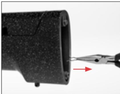
Use pliers to remove the comb retaining clip from the rear shaft of the comb.
