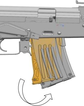
4. To load the magazine, place the round at the top (open end), push down and backwards making sure that the back of the cartridge is facing the rear of the magazine. Repeat this procedure until magazine is fully loaded (10 rounds). Tap the back side of the magazine against the palm of your hand to insure the proper alignment of the cartridges
