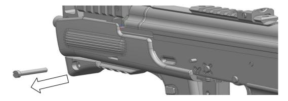
2. Move the hand guard's extension in the desired position
