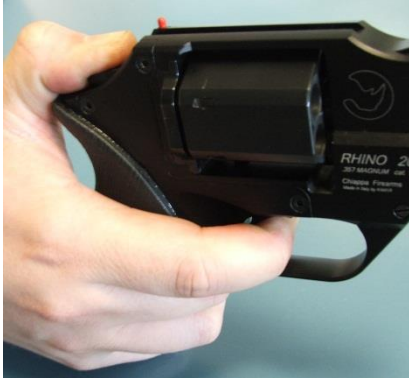
Figure 3: Releasing the external hammer
