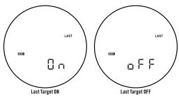
the Quick Set Menu by pressing and releasing the MODE button until the Last Target icon is shown in the upper right portion of the display. Press and release the POWER button to turn Last Target on/off. Press MODE to save the selection.
