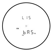
Internal display as seen through the RX-1400i TBR/W after the power button is pressed - Allows you to confirm the output settings or load that is actively selected in the rangefinder.
