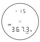
WIND will provide a fixed 10 mph full wind value, meaning it assumes the wind is at 90 degrees to the muzzle. We chose 10 mph as a way for the user to easily calculate corrections on the fly. If the wind is 5 mph, from the 3 o'clock or 9 o'clock position, the shooter would half the hold value. If the wind is 20 mph, the shooter would double the wind hold value. If the wind isn't
