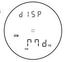
Press and release the POWER button to toggle between high, medium, and low. Press MODE to save the selection.
