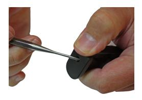
Next, remove the retainer plate, magazine spring, and follower from the magazine body.
