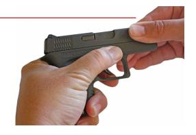
NOTE If the slide is pulled too far back it will reset the striker and will not slide forward off of the receiver. Do not use force! Repeat the previous steps.
