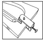
When in place, the stirrup is a clamp that provides a screw thread hanging below the handle for securing the MONOGRIP\* to the frame. No alternation of the firearm frame is needed. Remove the screw from the stirrup.
