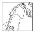
5 MONOGRIP\* should be guided up behind the trigger guard, then pivoted to cover the frame straps. The grip must mate with the semi-circular loops at the top of the gun handle. MONOGRIP\* must be fully seated on the frame before inserting mounting screw.
