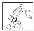
Your MONOGRIP® is designed to fit an average size firearm frame. However, frame dimensions do vary slightly from firearm to frearm. If necessary, your MONOGRIP® can be adjusted by placing small shim(s) of tape (as shown) on the lower corner of the front strap. Add or subtract tape until grip is flush with backstrap.
