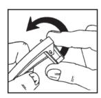
Place the stirrup over the bottom strap of the handle and rotate it until the hole in each side engages the stock pin.
