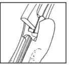
Mate the firearm handle and MONOGRIP® by first placing the stirrup and stock pin into the internal guide grooves using your thumb to spread the grip.
