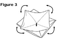
Continue around blind, pulling the hubs one at a time, until all hubs are extended as shown in Figure 5.
