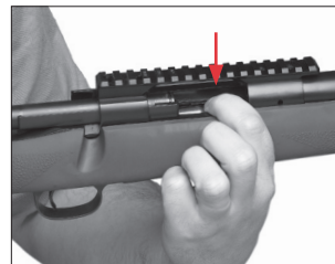
Hold down the top cartridge and close the bolt.
