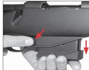
Press the ambidextrous magazine release and remove the magazine.
