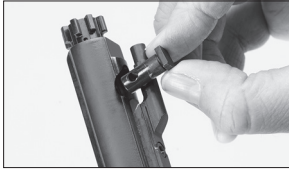
Rotate and remove the bolt cam pin.
