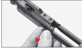
Remove the firing pin retaining pin.
