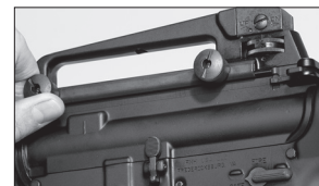
Properly installed carry handle. Do not over tighten the locking knobs.
