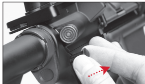
Withdraw the rear take-down pin from left to right.
