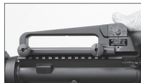
Rotate the carry handle on to the receiver from the right.
