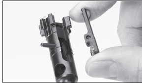
Remove the extractor from the bolt.
