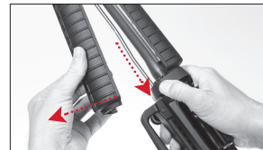
Press down on the handguard slip ring and remove one of the handguards.
