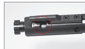
Align the cam pin hole with the cam pin slot.
