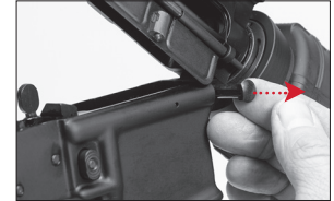
Withdraw the front take-down pin from left to right.
