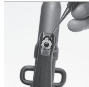
Use a punch or similar object to adjust the front sight post while zeroing.
