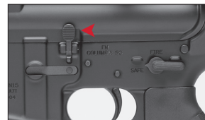
Press in on top of bolt release to release the bolt.
