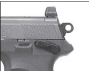
Hammer decocked for double-action firing and the "safety" in the on safe position.
