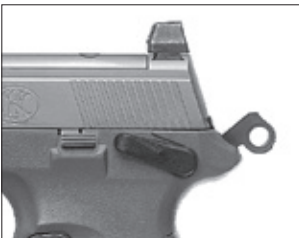
Hammer cocked for single-action firing and the "safety" in the on safe position.
