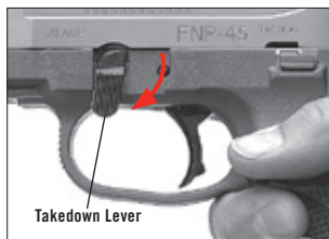
Rotate the takedown lever downward.
