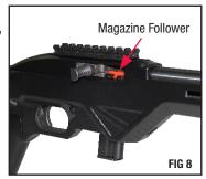
5. After inserting a new loaded magazine into the rifle (don't forget to first engage the manual safety) if the bolt is locked in its open position by the bolt lever, to chamber a cartridge, just pull bolt rearward and away from the receiver (in the opposite direction of the engraved arrow) and let the bolt move freely forward.
