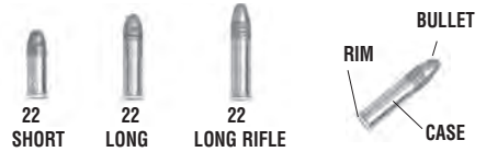
PICTURE 2 This picture shows the main parts of the ammunition. 22 CALIBER CARTRIDGE
