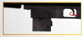
BE SURE THAT RIFLE IS POINTED AT TARGET! With action closed, move safety to "F" position. Pull trigger. To repeat, open and close action. The discharged shell will be ejected and a new cartridge will be fed into the chamber. Pull trigger. Repeat process as desired until magazine is empty.
