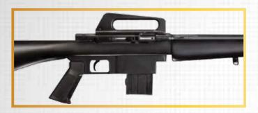
Draw safety on and insert a loaded magazine into the rifle. Retract bolt handle fully to the rear of the receiver slot and release. Allow the bolt to be snapped back under the full force of the operating springs. Bolt automatically picks up a cartridge from the magazine and feeds it into the chamber. Do not ease bolt forward.
