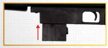
Position magazine open end up and ears rearward. Insert magazine into the opening of the trigger guard housing. Push magazine inward until it engages with the magazine catch.
