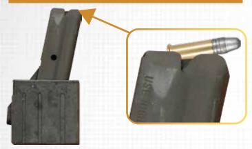
Hold the magazine box firmly with in one hand. With the other hand, position cartridge over magazine lip just forward of notch. Insert cartridge head under ears at rear of magazine. Repeat this procedure as derived or until the magazine is fully loaded to its capacity.
