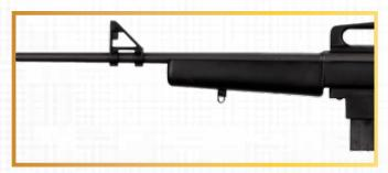
After firing, swab bore with clean cloth patch wet with approved cleaning solvent. Wipe dry. Apply light coat of oil on barrel bore, bolt and other metal surfaces to keep free of rust.
