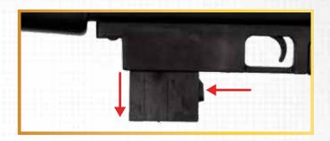
To disengage magazine, press magazine catch rearward, hold on lock and pull box downward and out.
