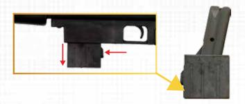
Draw safety on and release the magazine from guard. Work action several times to remove any cartridge left inside the chamber. Slide bolt handle rearward and lock piece. Inspect the chamber to make sure no cartridge is left. Empty magazine can be placed back if desired.
