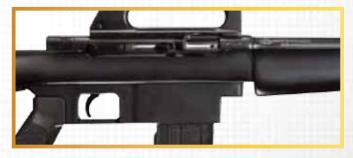
Safely lever is at right side of the receiver and rearward of the bolt operating handle. Pull safely latch towards the "S" mark engraved on the receiver. Trigger is locked up in the process and gun can no longer be fired.
