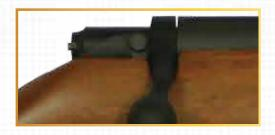
Pull safety on right side of the receiver in the direction of the "S" mark. This locks trigger and gun cannot be fired.
