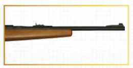
After firing, swab bore with clean cloth patch wet with approved cleaning solvent. Wipe dry. Apply light coat of oil on barrel bore, cocking cam, bolt and other metal surfaces to keep free of rust.
