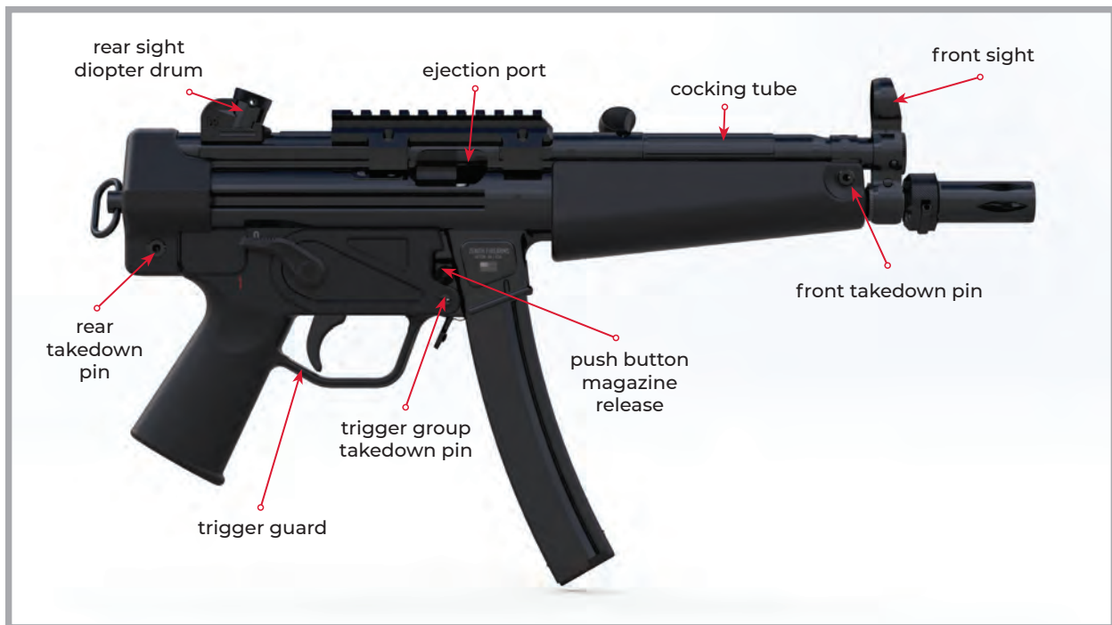
Figure 2: ZF-5 right side view
