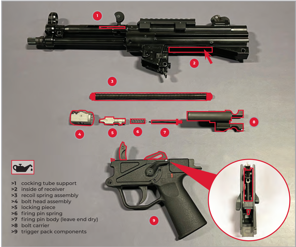
Figure 37: ZF-5 lubrication points
