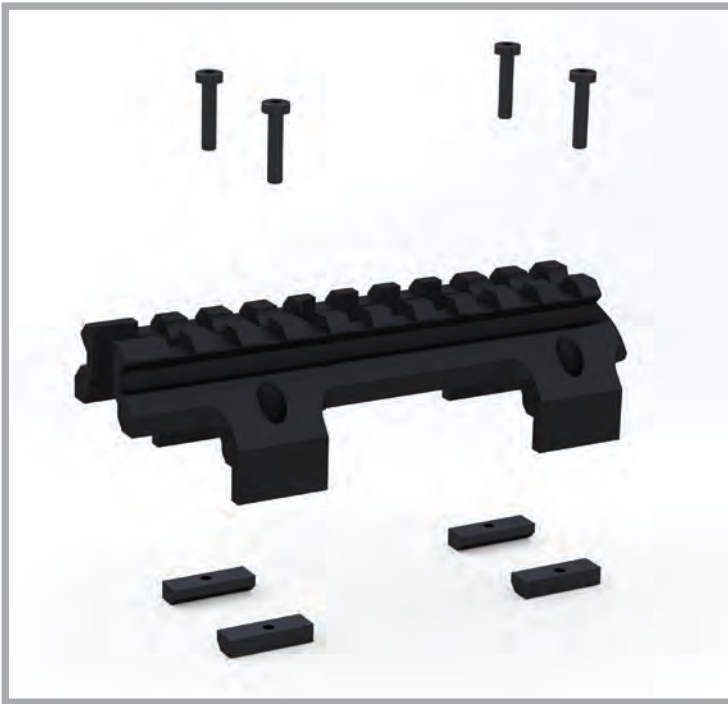
Figure 9: Mounting the Picatinny optic rail
