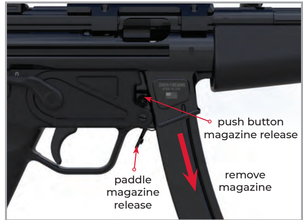
Figure 21: Removing the magazine
