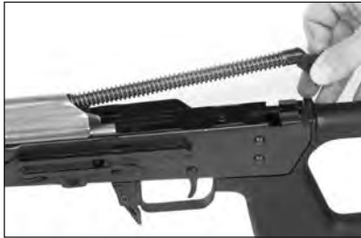
Fig. 13 - Taking out of the bolt recoil mechanism from the receiver ;
