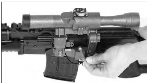
Fig. 10- Stripping of the optical sight;
