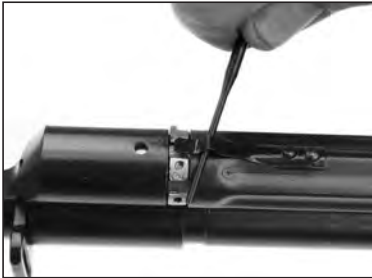
Fig. 6 - Lifting the spring securing pin
