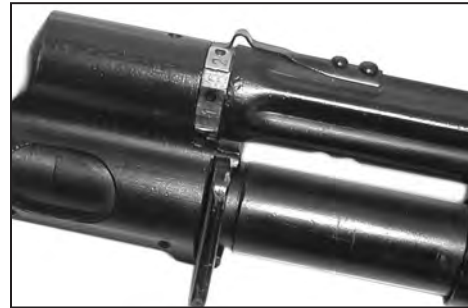
Fig. 7 - Regulator in position 2 - normal conditions
