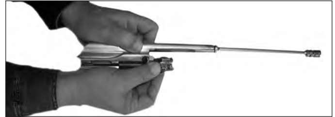
Fig.15 - Stripping of bolt with carrier and piston :
