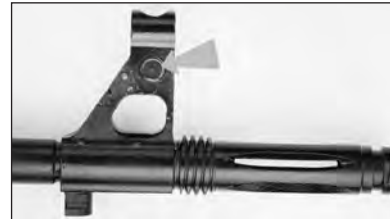
Fig. 20 - Moving the front sight post carrier
