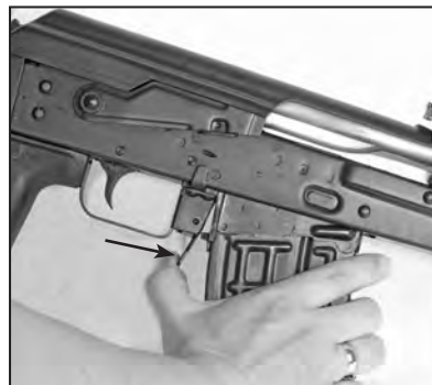
Fig. 11- Stripping of the magazine;
