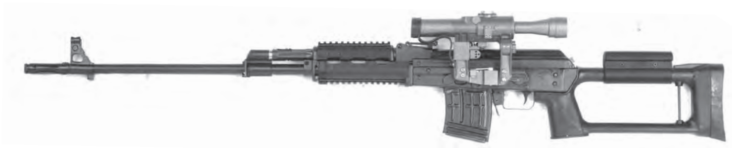
Fig. 1 - Semiautomatic sniper rifle M91 (the model of optical sight can vary depending on the customer's request)
