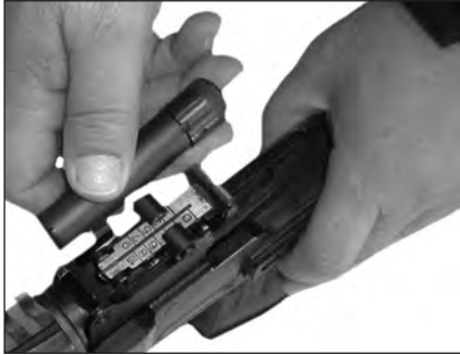
Fig.16 - Stripping of gas cylinder:
