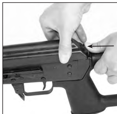
Fig. 12 - Stripping of receiver cover ;
