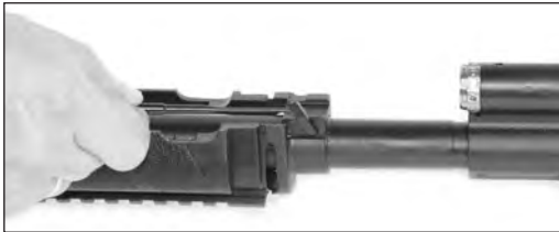
Fig.17 - Stripping of lower handguard
