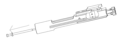
Push the bolt in towards the carrier until the bolt rotates and comes to a stop, then turn the bolt cam pin 90°.
