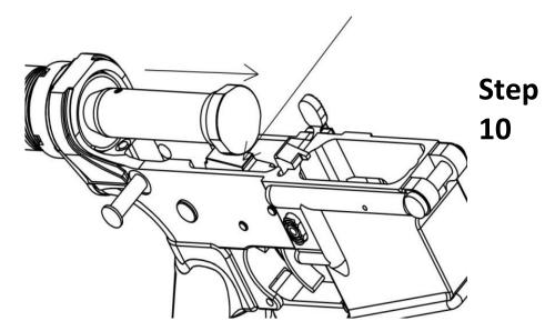
Depress the buffer retainer pin to permit the buffer and the spring to move forward. Depress the hammer to allow the spring and the buffer assembly to continue moving forward and be removed from the receiver extension.
