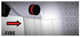
To move the safety to the FIRE position, push the safety button from right to left as far as it will go (See Above Drawing 2). A red ring around the safety button will be visible when the safety is in the FIRE position. If the trigger is pulled with the safety in this position, the gun will fire unless the unique Altor barrel safety is still in the SAFE position. In order to fire the firearm, both the button safety and the barrel safety (See page 7, photo 4) have to be in the FIRE position.
