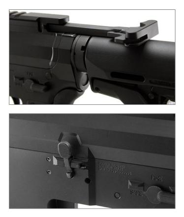
Pull the charging handle all the way to the rear and press the bottom portion of the bolt catch. Release the charging handle. This locks the bolt in the open position.
