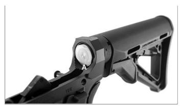
Press down on the buffer retainer (A) while holding the buffer back. Allow the buffer to travel forward slowly after clearing the retainer.
