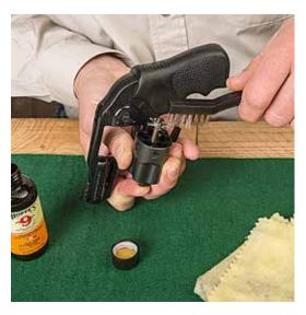
Use a bronze brush dipped in cleaner to scrub the back of the barrel, rear cylinder opening, cylinder faces and inner frame. Also scrub the extractor rod, the hammer face and landing.
