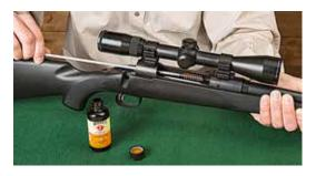
Working in a well-ventilated area, attach a bore brush to the cleaning rod and apply Hoppe's No. 9 Bore Cleaner. Run it through the barrel completely, then pull it back out again. Repeat three or four times to dislodge any powder and metal fouling.
