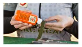
**STEP 2.** Apply a few drops of Hoppe's No. 9 Lubricating Oil to the Boresnake's tail.
