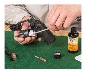
Follow the same procedure with each chamber of the cylinder. Next, attach the patch holder to the cleaning rod, apply cleaner and run it through the bore. Repeat until patches emerge clean. Run a dry patch through, apply a few drops of lubricating oil and make one final pass. Repeat the same step for the cylinder.
