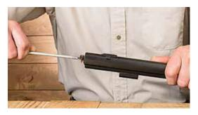
After two or three shots, apply Hoppe's No. 9 Black Powder Cleaner & Patch Lubricant to a bronze brush and run it down the bore and back.
