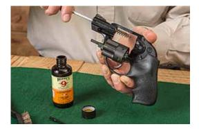
Apply Hoppe's No. 9 Bore Cleaner to a bore brush. Starting at the muzzle, run it through the barrel until it comes out the back side. Run it back out, and through again three or four times reapplying cleaner as needed.
