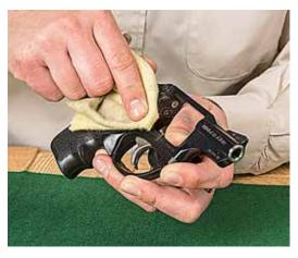
Finally, apply a few drops of lubricating oil to a cloth and polish all exterior metal. Switch to a Hoppe's Triple Threat Cloth and polish metal to a high luster.
