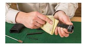
Inspect each part to make sure surfaces are spotless. Continue scrubbing with cleaner as needed until there are no deposits on any surfaces. Wipe down all parts with a clean, dry cloth. Apply a few drops of oil to a fresh cloth and polish all parts, wiping off any excess lubricant.
