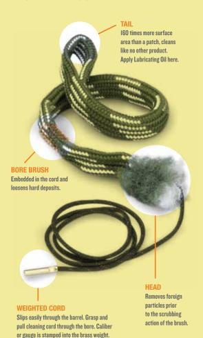
NOTE: BoreSnake for a 20-gauge shotgun. Mop head sizes vary based on caliber size.
