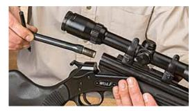
Most inline muzzleloaders can be disassembled for quick, easy cleanup between shots. Along with the same muzzlecleaning steps above, you may occasionally remove the breech plug to thoroughly clean the flash channel. This makes cleaning the bore much easier when done at the same time.
