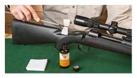
Remove the bore brush and attach a slotted patch holder. Insert a patch, apply bore cleaner and, starting at the breech end, push it through the bore one time. Do not pull it back through, as this will only redeposit debris that was removed. Replace the patch and repeat until the final patch comes out clean.
