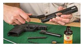
Dip a bronze brush in cleaner and scrub each part thoroughly. Take your time and work the bristles into hard-to-reach areas, reapplying cleaner as needed. Also clean the inside of the magazine well and dry off with a cloth. Avoid getting cleaner on the grips.
