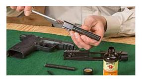
Apply Hoppe's No. 9 Bore Cleaner to a bore brush and run it through the barrel until it comes out of the opposite end. Repeat this process three or four times, reapplying cleaner as needed.
