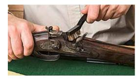
Once you are finished shooting for the day, it's a good idea to clean the flash channel. Use a hand-held bronze brush dipped in the bore cleaner to clean and scrub the nipple and hammer, or in the case of a flintlock, the frizzen and pan, and surrounding areas.
