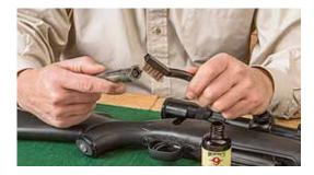
With the bore clean and properly lubricated, apply Hoppe's No. 9 Bore Cleaner to a hand-held bronze brush and thoroughly scrub down the bolt and all internal surfaces. Take your time and let the bristles work the cleaner into hard-to-reach places.
