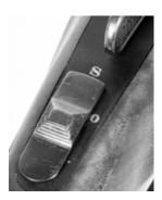
Barrel Selectors – The "O" (over) and the "U" (under) located next to the selector switch are for training purposes only. The selector must be moved fully to either the left or right and must never be set in between these settings as damage to the safety mechanism and/or selector switch can result.
