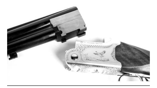
Swing the barrel up firmly without forcing to its fully closed position. The lever will snap to a centered position. The barreled action is now ready to receive the forearm.
