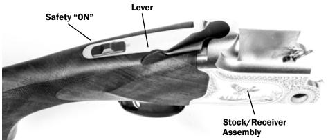
The stock/receiver is now ready to accept the barrel assembly. To assemble the barrel to the stock/receiver assembly, locate the half-round cuts in the barrel lug and the round hinge pins inside of the receiver. With the barrel assembly held approximately 45 degrees to the stock/receiver assembly, mate the round cuts of the barrel assembly to pivot on the round receiver hinge pins.
