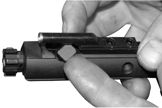
10. Remove cam pin by lifting it out away from bolt and carrier.
