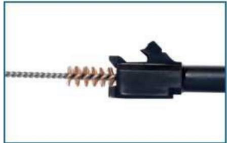
4. Lightly dampen the microfiber brush with gun oil or lubricant and push it through the barrel from the chamber end to lightly oil the barrel.
