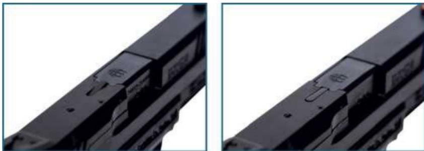
The BRG9 Elite includes a loaded chamber indicator. The loaded chamber indicator will be raised above the barrel when a cartridge is in the chamber.
