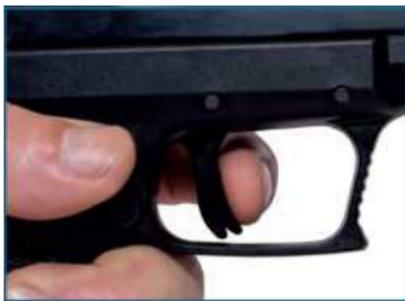
The BRG9 Elite includes a trigger safety. The trigger safety is a lever incorporated into the trigger. The trigger safety will prevent the trigger from being pulled unless the trigger safety is fully depressed. It is designed to prevent the firearm from firing if it is dropped or the trigger is accidentally depressed from the side.
