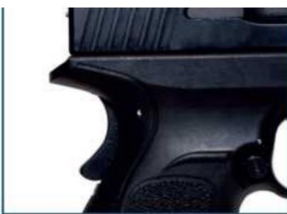
The BRG9 Elite includes a grip safety. The grip safety is located at the top rear of the pistol grip. The firearm is designed not to fire unless the grip safety is fully depressed. The slide cannot be pulled to the rear unless the grip safety is deactivated.
