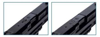
The BRG9 Elite includes a loaded chamber indicator. The loaded chamber indicator will be raised above the barrel when a cartridge is in the chamber.
