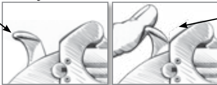
Rebounding Hammer NORMAL Half-Cock Position
