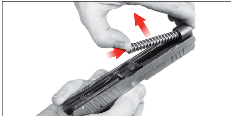
Figure 23 — Removing the recoil spring assembly. Caution: spring under tension!
