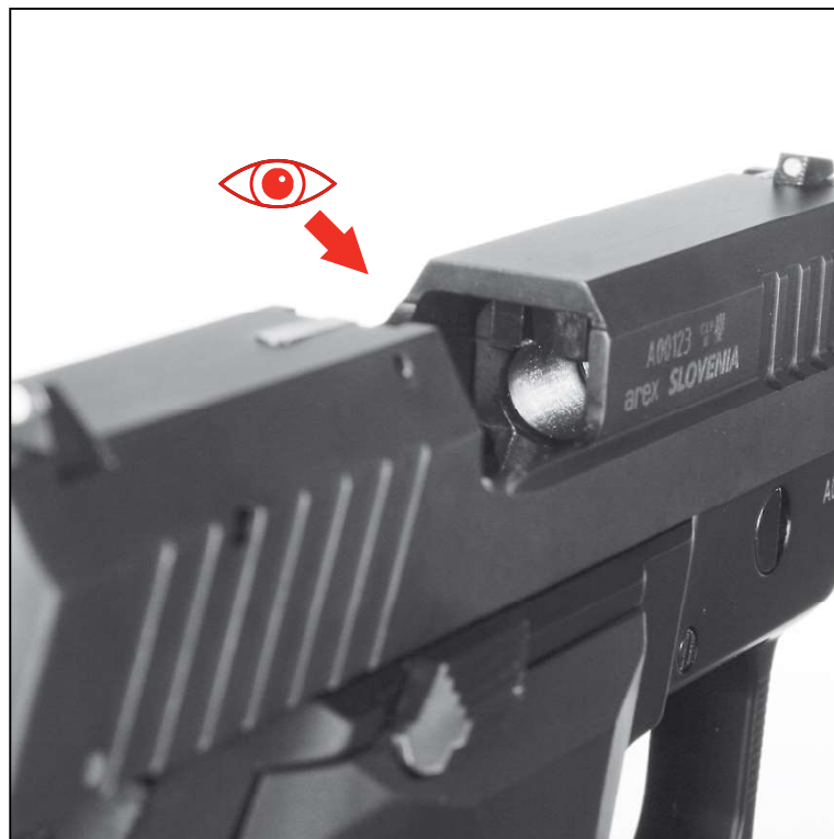
Figure 6 — inspect chamber and magazine well
