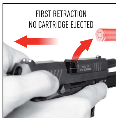
Figure 18 Briskly retract slide once: watch for ejected cartridge
