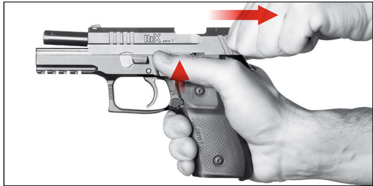
Figure 5 — fully retract slide TWICE
