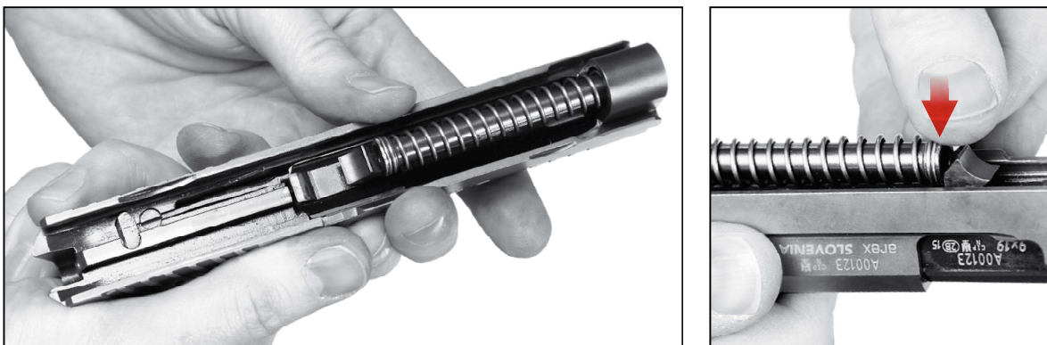
Figure 29 — Reassembling the recoil spring onto the barrel and slide (wide end of the spring guide located in front of barrel's guiding lug)
