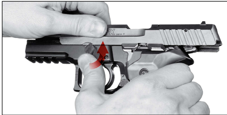
Figure 31 — Pivot the disassembly lever counter clockwise
