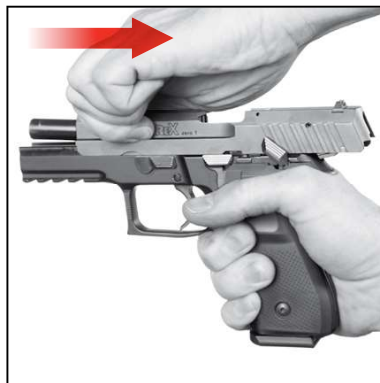
Figure 11 Use front serrations to retract slide if safety is engaged
