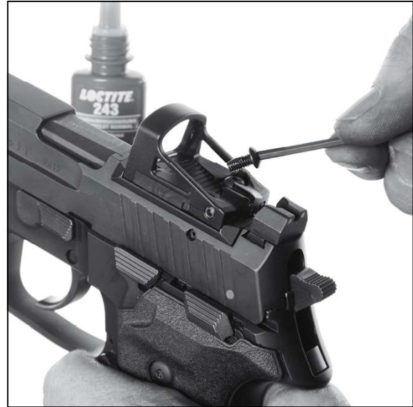
Figure T4- Mount the reflex optical sight according to manufacturer's instructions
