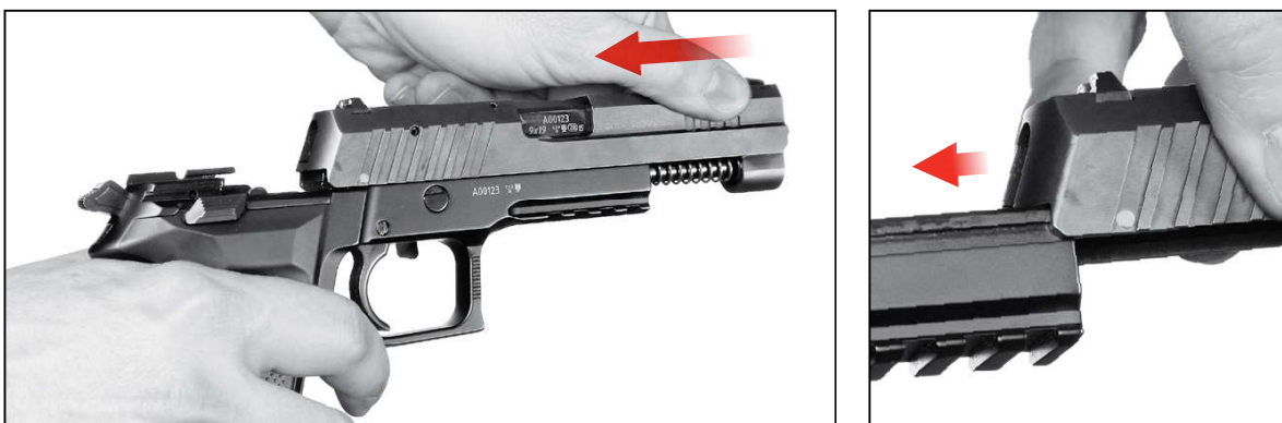
Figure 30 — Mounting the slide on the frame (frame guides aligned with slide grooves)
