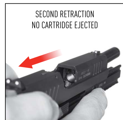
Figure 19 Retract and hold slide back again: verify empty chamber
