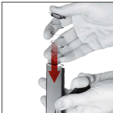
Figure 32 Insert the follower, spring, and locking plate
