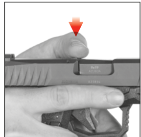
Figure 15 Checking the loaded chamber indicator tactilely
