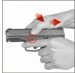
Figure 43 Push the slide down and pull it back seeing the disassembly latch spring up
