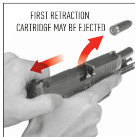
Figure 21 Briskly retract slide once: watch for ejected cartridge
