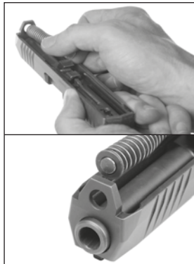
Figure 39 Inserting the stepped end of the recoil spring assembly into the front of the slide
