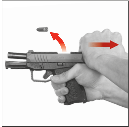
Figure 5 — retract slide: watch for ejected cartridge
