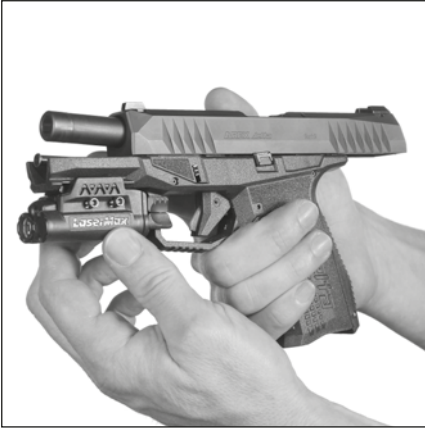
Figure 53 — Installing accessory weapon light/ laser module onto the rails
