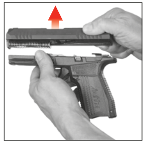
Figure 25 Lifting the slide from the frame
