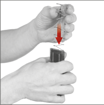
Figure 44 — Insert the follower and spring
