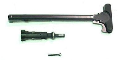
6. Inspect the charging handle for cracks, bends or breaks.
