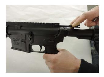
4. Place the safety on "FIRE". Squeeze the trigger and hold the trigger to the rear; the hammer should fall. Pull the charging handle to the rear and release it. Release the trigger. You should hear a click as you release the trigger. Squeeze again; the hammer should fall.
