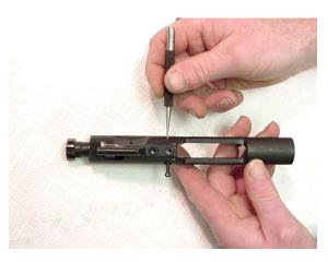
4. Move the bolt assembly forward to the unlocked position and remove the firing pin retaining pin. Do not open or close the split end of the firing pin retaining pin.
