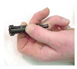
9. Press the rear of the extractor to check that the spring works.
