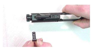
6. Insert the cam pin and give it a ¼ turn. (Firing your rifle without the cam pin installed will result in the destruction of the rifle and possible injury.)
