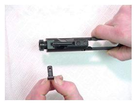
7. Give the bolt cam pin a ¼ turn and lift it out.
