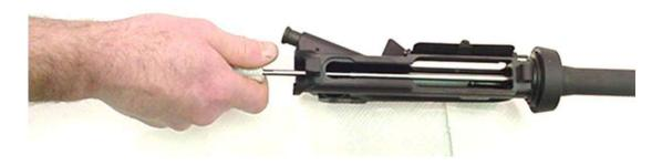
2. Install the chamber brush on the cleaning rod, dip it in cleaning solvent, and insert it into the chamber and locking lugs. Clean by pushing and twisting the cleaning rod.
