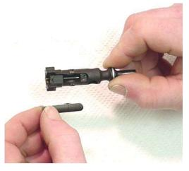
11. Remove the extractor and spring assembly. Do not remove the spring assembly, its plunger or the O-ring from the extractor.
