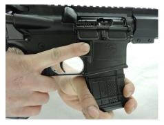
2. **Remove the magazine** by depressing the magazine catch button and pulling the magazine down.
