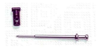
9. Inspect the bolt cam pin for cracks or chips. 10. Inspect the firing pin for bends, cracks, or a sharp, chipped, or blunted tip.
