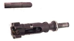
5. Press the ejector in repeatedly to remove accumulated brass shavings from the ejector hole and assure the ejector moves freely. Lubricate it generously.
