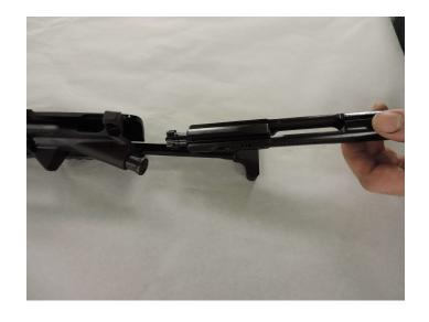
11. Slide the bolt carrier assembly, bolt extended, into the upper receiver.
