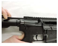
2. Release the charging handle. If the bolt carrier doesn't fully close, tap the forward assist to close it.
