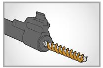
Bore brush loosens built-up fouling in rifle & handgun bores
