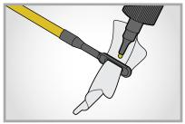
Use slotted patch tip to apply solvent to bore
