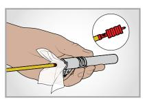
Use dry patches with jag to remove loosened fouling from bore
