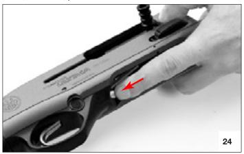
Use the cocking handle to retract the breech bolt until it snaps into the open position.
