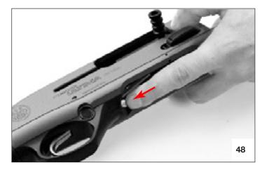
Remove the trigger guard retaining pin by pressing with a pin punch or an awl.
