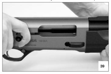
Unscrew the front cap of forend in a counterclockwise direction.
