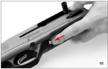
Use the cocking handle to retract the breech bolt until it snaps into the unlocked position.
