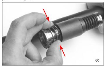
Check that the carrier stop push button is pressed all the way down. If it is not, push it all the way down.
