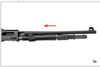
Slide the forend into place over the gas cylinder/the valve assembly and magazine tube checking for the correct centering on the receiver face.
