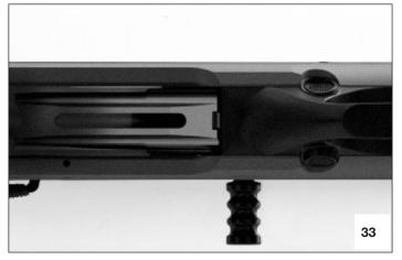
Pull back the breech bolt to extract and expel the live cartridge from the chamber.
