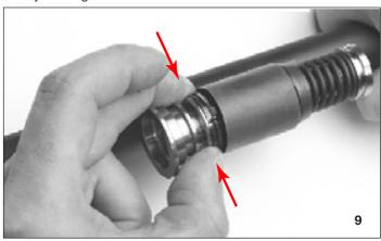
Check that the carrier stop push button is pressed all the way down; otherwise, push it down.
