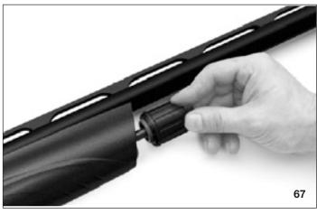
Keeping your fingers away from the ejection port, press the breech bolt release button and gently guide the breech bolt to lock.
