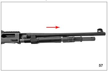
With the barrel assembly off the forend adapter/piston stop can now be removed.
