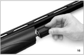
Keeping your fingers away from the ejection port, press the breech bolt release button and gently guide the breech bolt to the lock position.
