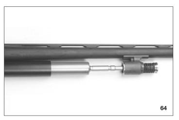
Slide the forend into place over the gas cylinder/the valve assembly and magazine tube, checking for the correct centering on the receiver face. The forend is in the correct position when it is fully against the receiver.
