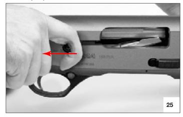
Engage the manual safety by pressing the safety button to hide the red ring.
