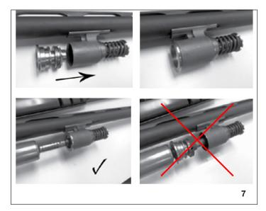
If the piston is mounted on the magazine tube shaft, remove it and insert it into the cylinder of the barrel, making sure to tighten the elastic seal with your fingers to facilitate insertion of the piston into the cylinder.
