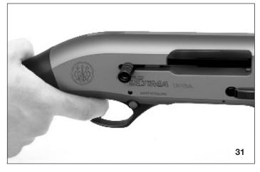
Engage the safety (red ring not visible), and if necessary, reload the shotgun according to the previous instructions.
