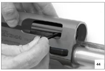
Over a flat surface, with the ejection port pointed upwards, slide the connecting rod with sleeve forward off the magazine tube shaft to extract the breech bolt assembly from the receiver.
