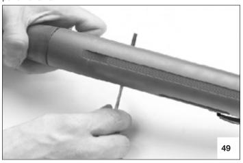
Keeping the breech bolt release button pushed all the way down, remove the trigger plate from the receiver using the trigger guard as a lever, first in the direction of the barrel and then outward.
