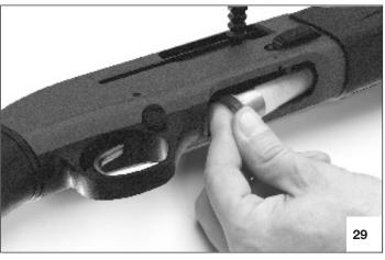
To fire, disengage the safety (red ring visible) and pull the trigger.
