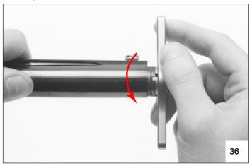
Remove the choke tube from the muzzle of the barrel.
