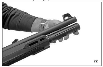
Install the barrel to mag tube clamp. Tighten the (2) hex screws securely.
