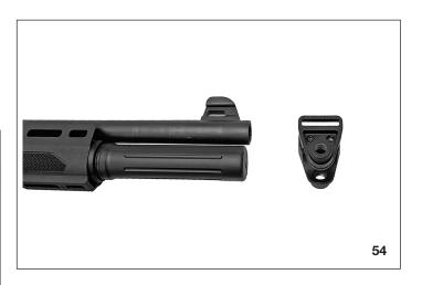
Unscrew and remove the mag tube cap.
