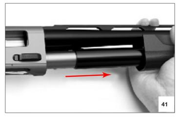
Pull the barrel out of the stock-receiver assembly while holding the piston inside the gas cylinder of the barrel.
